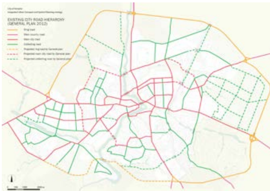
Figure: Existing road hierarchy with many main roads. Structured hierarchy is barely visible at all.
