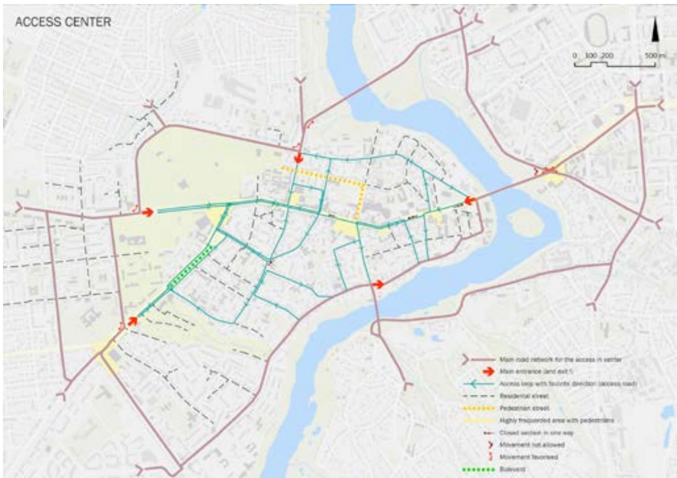
Figure: Access to City centre with loop system for private motorised transport
