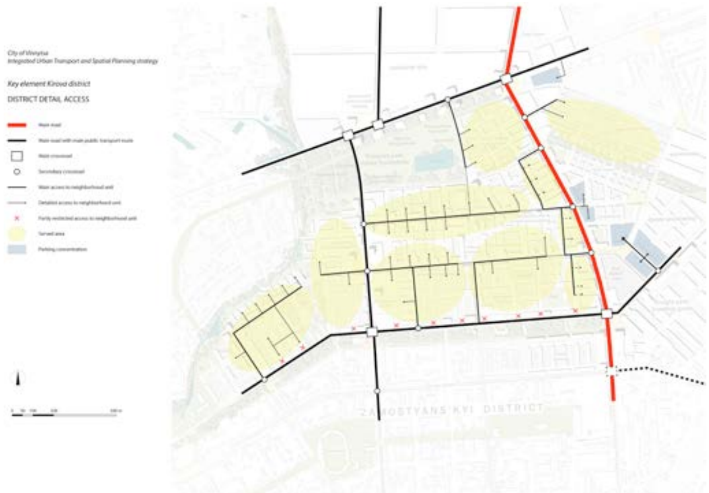
Figure: Access principles for private transport. Access roads and loops create pockets, which are free of through-traffic
