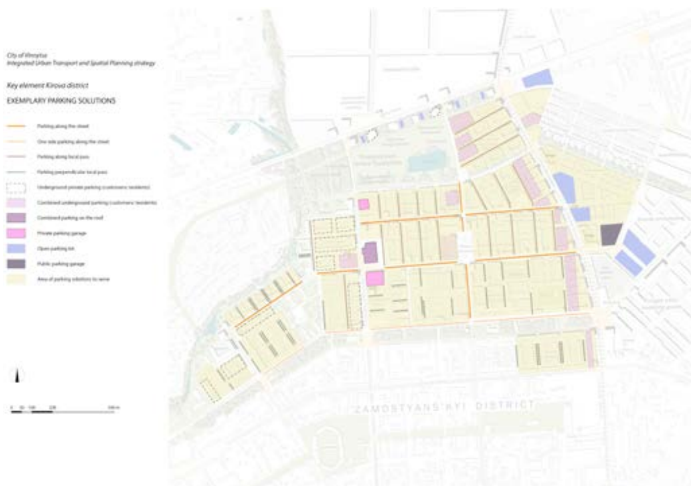
Figure: Principles for location of private and public parking. Various solutions, no parked cars in courtyards!
